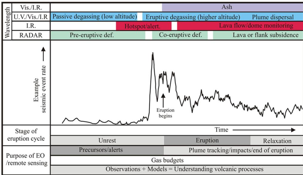
**Fig. 1.** An illustration of some of the applications of remote-sensing techniques to a volcano during a hypothetical eruption cycle. The example seismic trace is intended to be schematic and is based on the number of seismic events per hour with magnitudes  $>3.2$ , 20 March–28 May 1980 at Mt St. Helens. (Robert Tilling) from GVN monthly reports Mount St Helens 05/1980 (SEAN 05:05) <http://www.volcano.si.edu/world/volcano.cfm?vnum=1201-05-&vpage=var>
