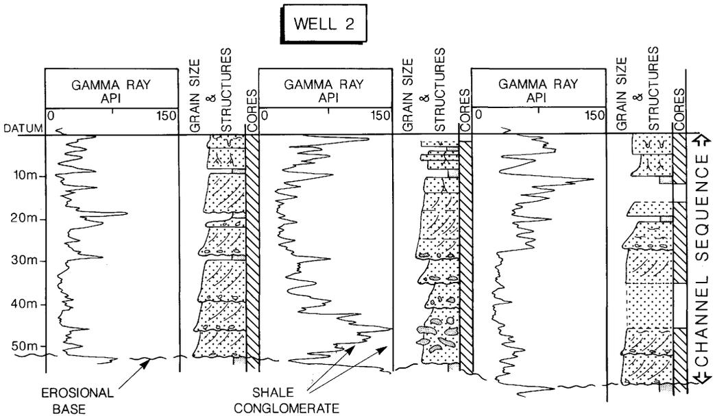
Fig. 6. Channel sandstone sequence across three wells with an interval of high gamma-ray values in Well 2 due to the presence of shale conglomerate.
