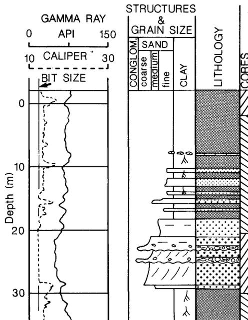
Fig. 4. Arkosic sandstone with an average 25% feldspar content (10% potassic) with a gamma-ray value similar to the surrounding silty shales.
