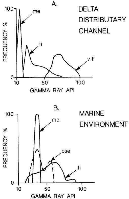
**Fig. 9.** Gamma-ray log values compared to sandstone grain size classes. A: Alluvial delta distributary sandstone. B: Winnowed marine sandstone. (from Simon-Brygoo 1980).
