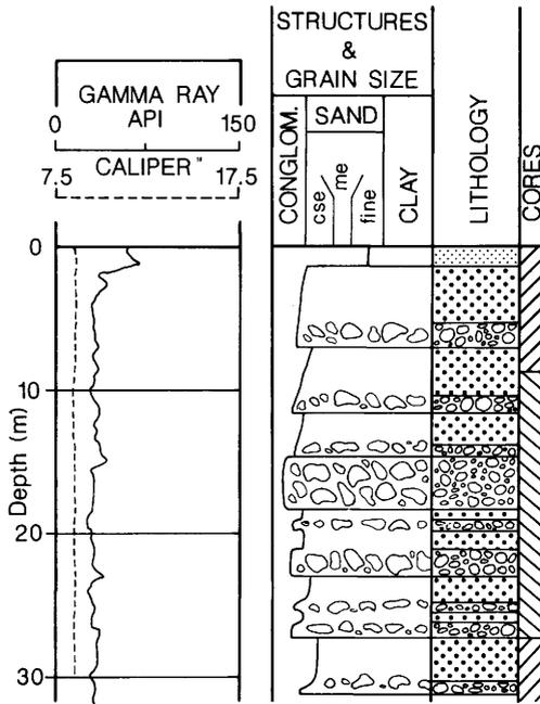
**Fig. 11.** Lack of correlation between gamma-ray log response and grain size variation in a very coarse grained sequence deposited by turbidity currents.
