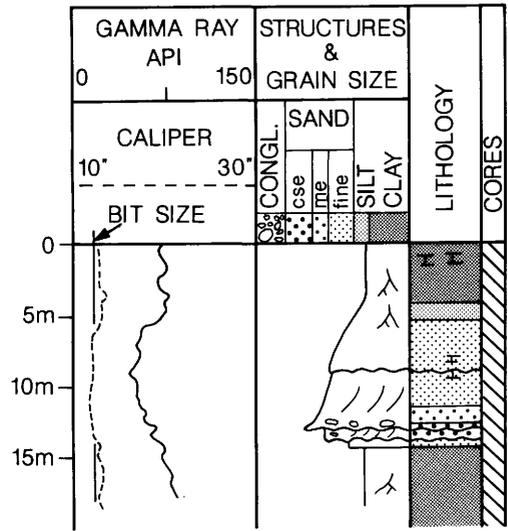
**Fig. 12.** Fining-upwards fluvial sequence with no bell shaped gamma-ray log.
