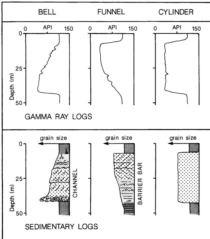
Fig. 1. The three principal gamma-ray log shapes and their corresponding sedimentary interpretation (after Serra & Sulpice 1975).
