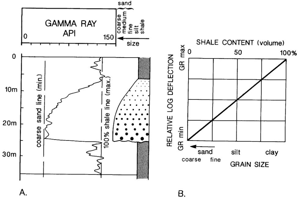
Fig. 2. Schematic representation of the use of the gamma ray log in facies analysis. A. Grain size changes reflected in the gamma ray log. B. Graphical presentation of the semi-quantitative relationships implied (modified from Rider 1986).
