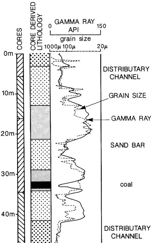
**Fig. 8.** Very close relationship between gamma-ray log values and core-measured sandstone grain size from a deltaic environment (from Simon-Brygoo 1980).
