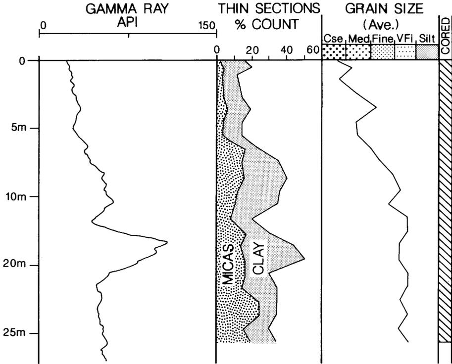
Fig. 5. Gamma-ray log in a sandstone with both radioactive grains (micas) and detrital clays. The micas vary more regularly with overall grain size than the clays.
