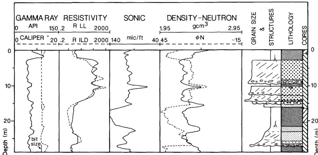
**Fig. 13.** Two sand bodies with a full set of corresponding logs. Lithological and textural information can be interpreted from each, especially the neutron density.
