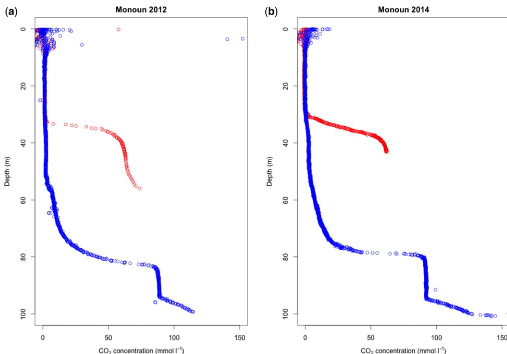
**Fig. 6.** Vertical profile of total CO<sub>2</sub> concentration estimated by SS change at Lake Monoun in (a) 2012 and (b) 2014. The fifteen measurements in 2012 and six measurements in 2014 presented in Table 2 are plotted together.
