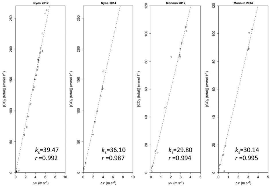
**Fig. 3.** Correlation between the change in SS and the total CO<sub>2</sub> concentration of lake water with Pearson's  $r$  at P06 of Lake Nyoos and at MRaft of Lake Monoun. The value of  $k_s$  is the slope of the regression line.
