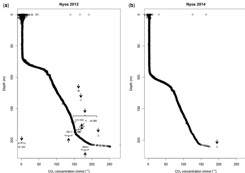
**Fig. 5.** Vertical profile of total  $\text{CO}_2$  concentration estimated by SS change at Lake Nyos in (a) 2012 and (b) 2014. The twenty-nine measurements in 2012 and seven measurements in 2014 presented in Table 1 are plotted together. Some measurements have anomalous values, which are indicated by arrows at the bottom of each measurement.
