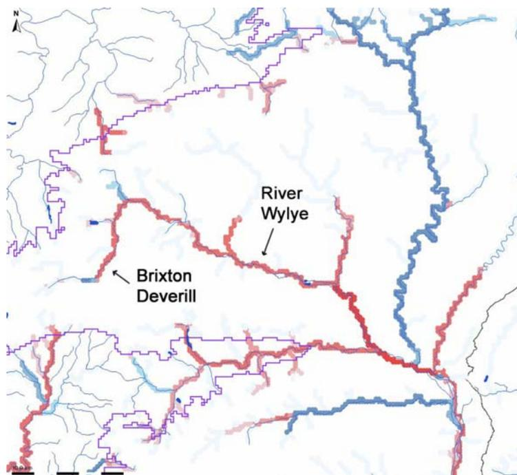
**Fig. 6.** Abstraction impact at high flows on the River Wylie; red cells show that, with the augmentation scheme off, the flow is now less than in the naturalized model run.
