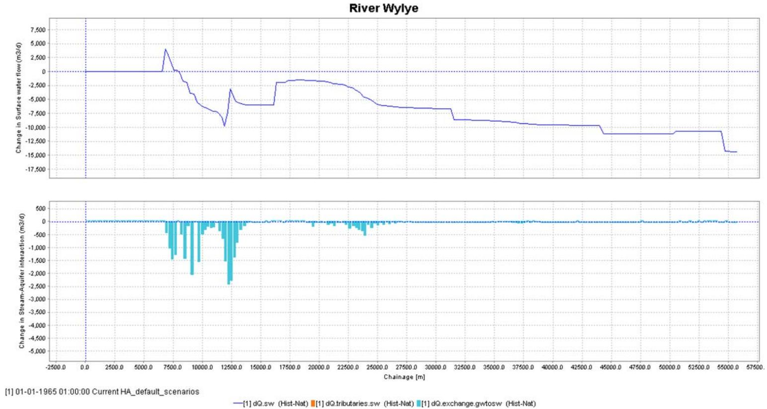
**Fig. 8.** Accretion profile at high flows of the River Wylfe, flow accretion above, groundwater–surface water interaction below. Augmentation scheme off.
