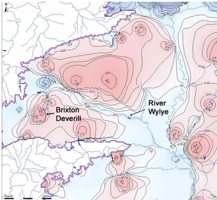
**Fig. 9.** Groundwater level difference plot (historic – naturalized) showing impact of groundwater abstractions and discharges in the Wylye catchment.
