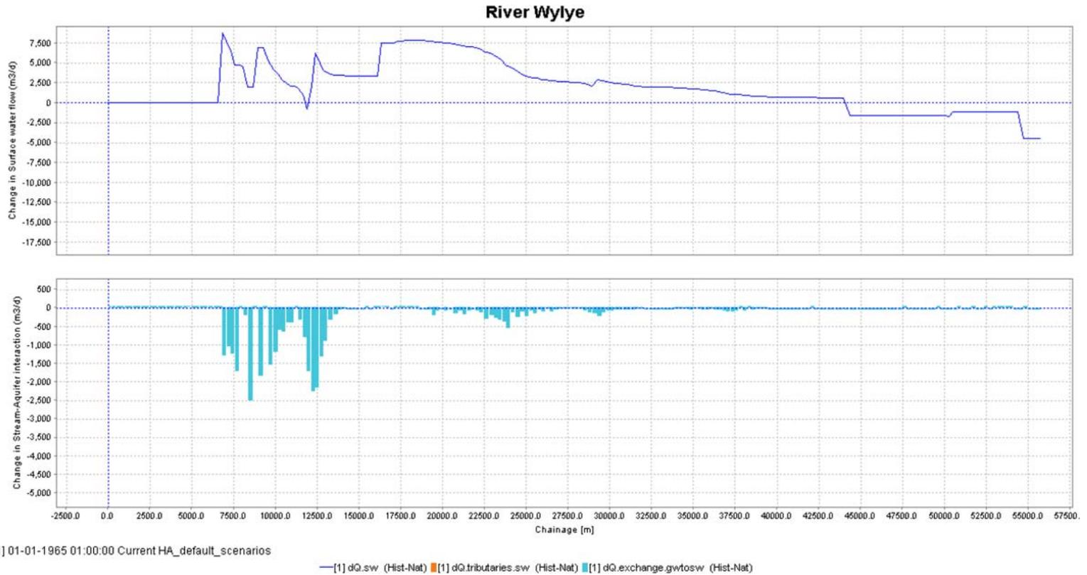
Fig. 7. Accretion profile at low flows of the River Wylie, flow accretion above, groundwater–surface water interaction below. Augmentation scheme on.
