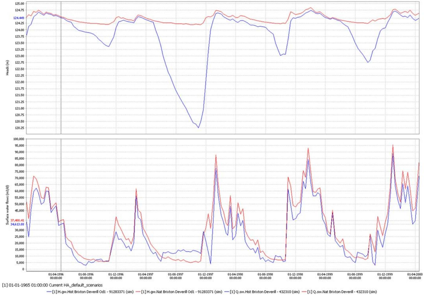
Fig. 3. User-defined NGMS graph showing groundwater heads and surface water flows for two model scenarios (historic and naturalized).
