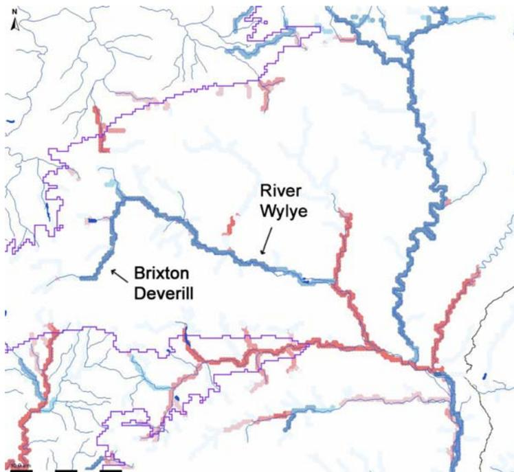
**Fig. 5.** Abstraction impact at low flows on in the River Wylfe; blue shows model river cells where anthropogenic influence (i.e. the augmentation scheme on the Wylfe) have increased flows above those of the naturalized model run.
