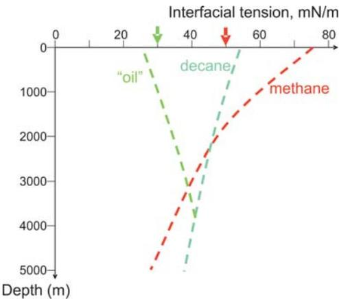
**Fig. 9.** Some published estimates of the variation of hydrocarbon–water interfacial tension with respect to depth (pressure & temperature conditions). The methane & decane curves indicate experimentally-measured trends from Firoozabadi & Ramey (1988). The ‘oil’ values are from Nordgård Bolås *et al.* (2005), constructed from empirical equations of Firoozabadi & Ramey (1988). Arrows show typical industry default values for oil–water (green) and gas–water (red) (d’Onfro, pers. comm., 2007).
