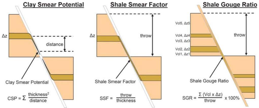
Fig. 3. The three main fault-seal algorithms. After Yielding *et al.* (1997), redrawn by Jolley *et al.* (2007).
