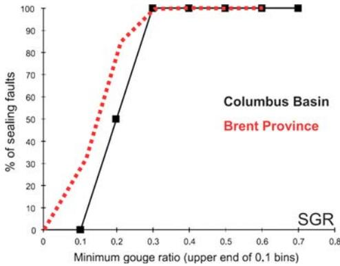
**Fig. 7.** Two subsurface calibrations of Shale Gouge Ratio. Black line summarizes calibration data from 12 reservoirs along 7 faults in Mahogany field, Columbus Basin, offshore Trinidad (from Gibson & Bentham 2003). Red line summarizes data from 29 faults in 15 fields in the Brent Province (from Yielding 2002).
