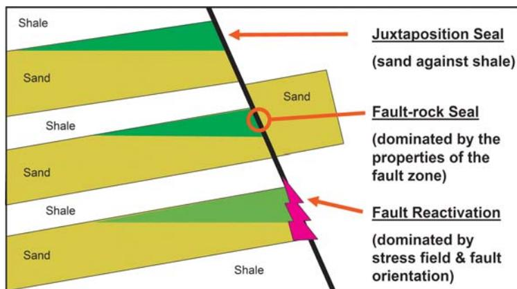
**Fig. 1.** Cartoon to illustrate the three critical factors for a viable fault seal: juxtaposition seal, fault rock seal, and *in-situ* stress state.
