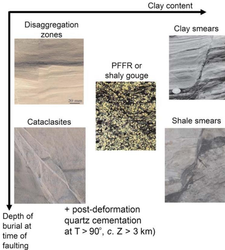
**Fig. 2.** Schematic plot to illustrate the main fault rock types generated in siliciclastic sequences. The axes represent 2 of the 3 main controls (clay content, and stress conditions during faulting); the third main control is post-faulting temperature history. Photographs from Lindsay *et al.* (1993), Fristad *et al.* (1997), Fossen & Gabrielsen (2005), van der Zee & Urai (2005), Fossen *et al.* (2007).
