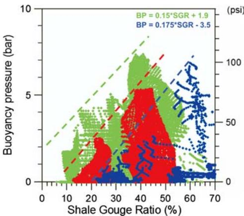
**Fig. 12.** Linear plot of the same data as that shown in the left-hand plot of Figure 11. Data points are coloured by maximum burial depth, blue <3 km, red 3–3.5 km, green >3.5 km. Note that linear seal-failure envelopes are consistent with the data distribution.
