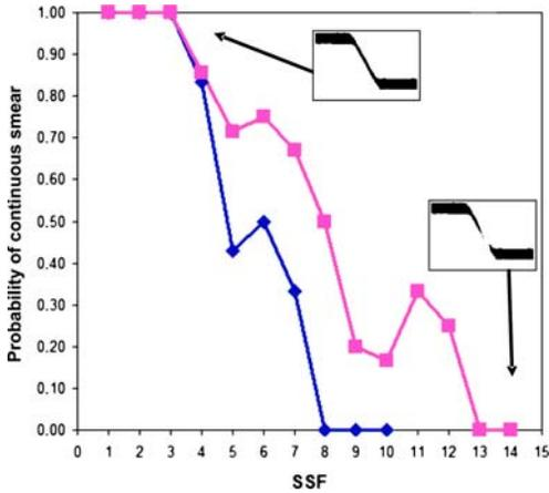
**Fig. 5.** Two calibrations of Shale Smear Factor (SSF). The curves show the observed probability of a smear being continuous from upthrown to downthrown side in cross-section view, at various different values of SSF (throw/thickness, Fig. 3). The blue curve summarizes deformation of laboratory samples (Takahashi 2003); the magenta curve summarizes outcrop observations by Childs *et al.* (2007).
