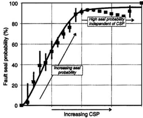
**Fig. 6.** Subsurface calibration of Clay Smear Potential (CSP) published by Fulljames *et al.* (1997). The data for this calibration were gathered on 91 reservoirs along 10 faults in three different fields (Niger Delta). (No scale on horizontal axis in original figure.)
