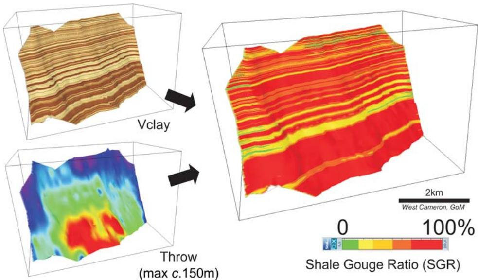
Fig. 4. Example of a subsurface fault-seal model. The fault surface was interpreted on 3D seismic reflection data (West Cameron area, Gulf of Mexico). Upper left diagram shows the sand-shale pattern mapped onto the upthrown side of the fault from well curves ( $V_{shale}$ ). Lower left diagram shows the displacement pattern mapped on the fault surface (from horizon offsets). Right diagram shows calculated distribution of shale gouge ratio (SGR) (equation in Fig. 3).
