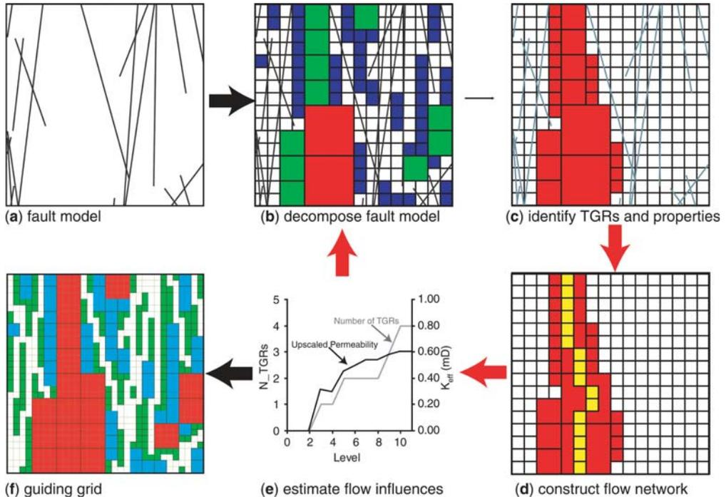
**Fig. 8.** An adaptive procedure for constructing a guiding grid for a fault model. Cells of different sizes and colours in (b) and (c) correspond to different decomposition levels. The images shown do not represent the final decomposition, since that produces cells that are too small to distinguish at the scale required to show the whole model in this printed page.
