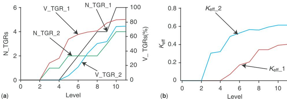
**Fig. 9.** N\_TGRs, V\_TGRs and the upscaled permeability,  $K_{\text{eff}}$ , along the vertical direction as a function of the subdivision level, respectively. Faults are assumed to be impermeable for this suite of models. Note that # indicates the model numbers.
