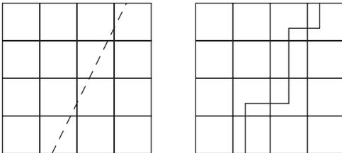
**Fig. 2.** Illustration of transformation of a fault into a staircase effective fault.
