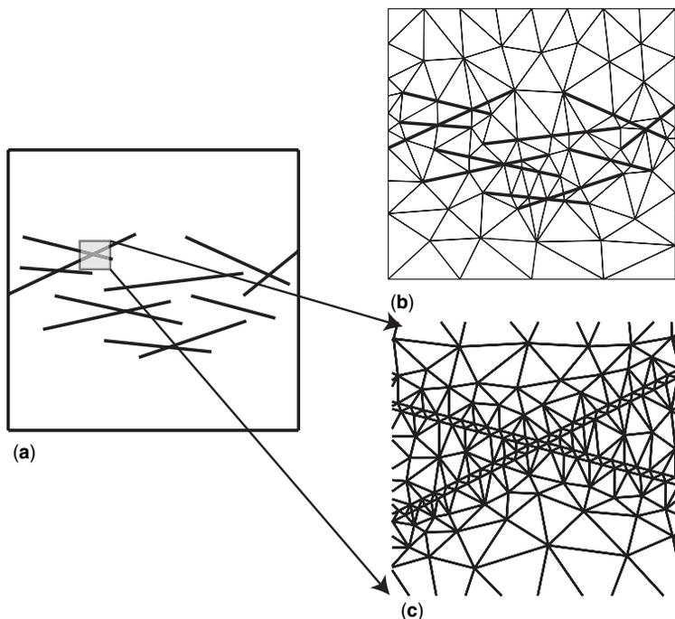
**Fig. 4.** A fault model and grids generated using IDF and EDF. (a) a simple fault model; (b) a geometrical grid generated by IDF for the whole model, where faults are shown as thick lines; and (c) a part of a grid generated using EDF corresponding to the indicated portion of the fault model in (a). From Ma *et al.* (2006).
