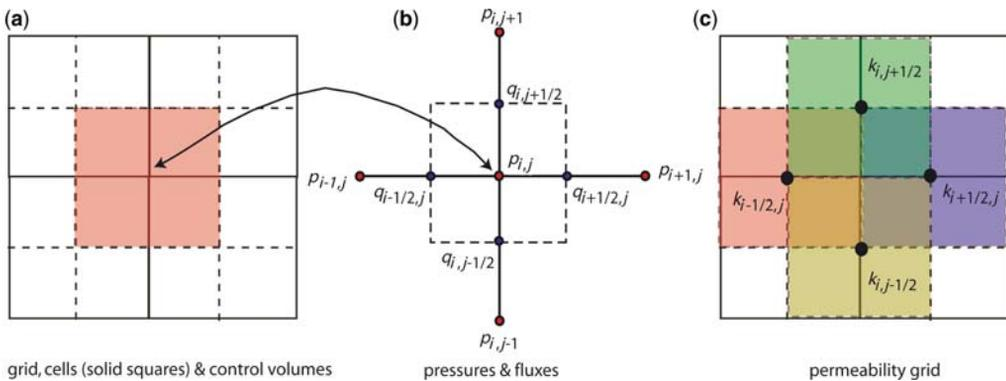
**Fig. 1.** Illustration of DDFM control volume finite difference scheme. (a) grid cells (divided by solid lines) and control volumes (divided by dotted lines); (b) discrete pressures (red) and fluxes (blue); (c) permeability grid.
