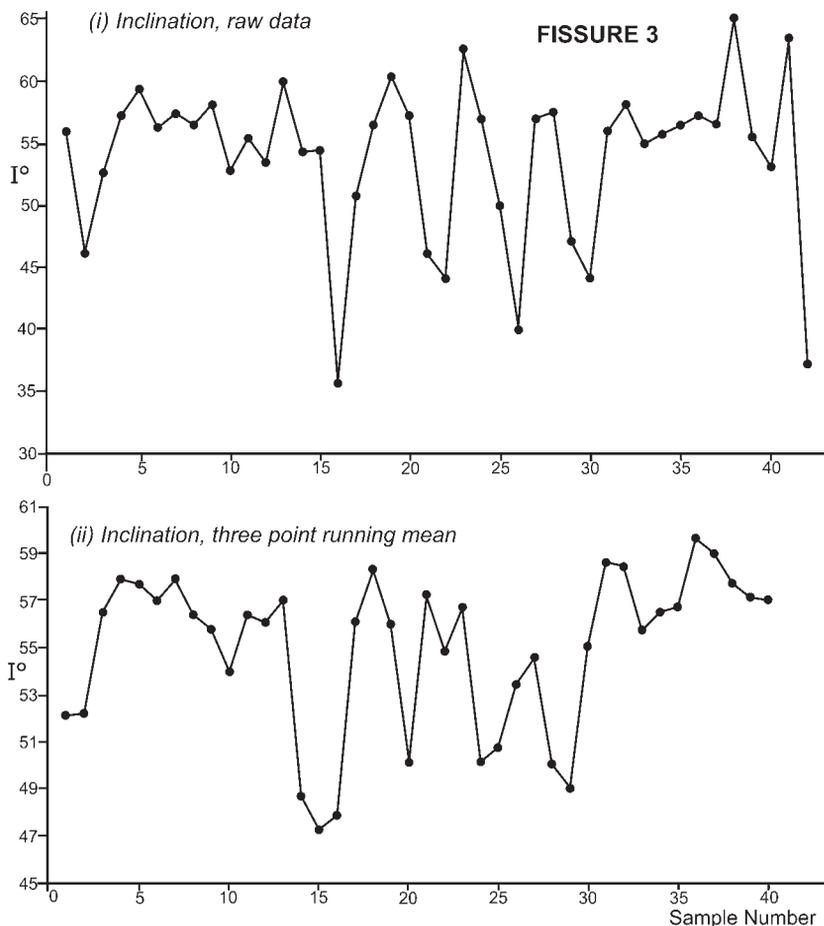
**Fig. 11.** Variation of the magnetic inclination recorded by travertine growth across fissure 3. Raw data and Fisherian means derived from applying a three-point filter are shown for comparison.
