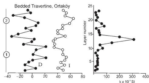
**Fig. 12.** Variation of magnetic declination and inclination derived from palaeomagnetic study of 24 successive layers through bedded travertine in the Ortaköy geothermal field. Also shown is the variation of magnetic susceptibility through this succession.
