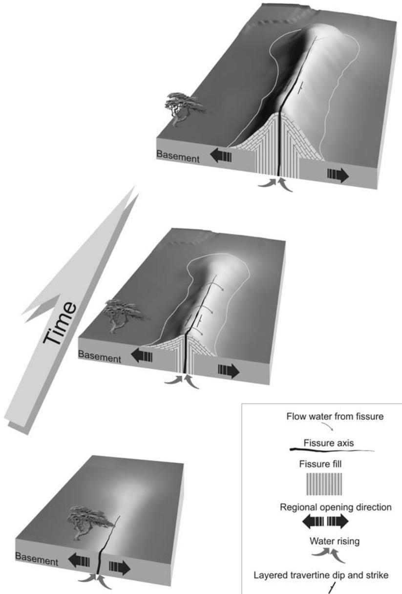
Fig. 1. The mode of formation of a travertine mound above an extensional fissure (after Mesci 2004).
