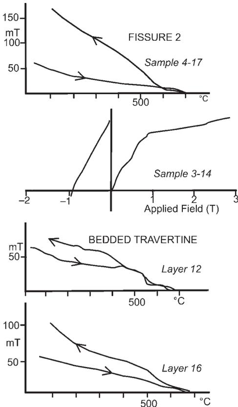
**Fig. 4.** Typical thermomagnetic (saturation magnetization ( $M_s$ ) v. temperature) determinations and IRM acquisition curves for samples of fissure and bedded travertine.
