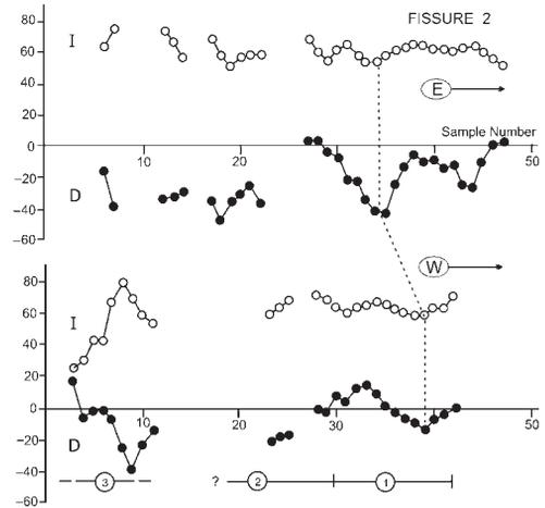
**Fig. 8.** Variation of the magnetic declination and inclination recorded by travertine growth across fissure 2.
