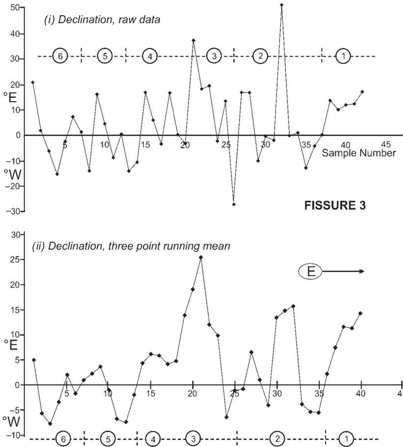
**Fig. 10.** Variation of the magnetic declination recorded by travertine growth across fissure 3. Both raw data and Fisherian means derived from applying a three-point filter are shown.
