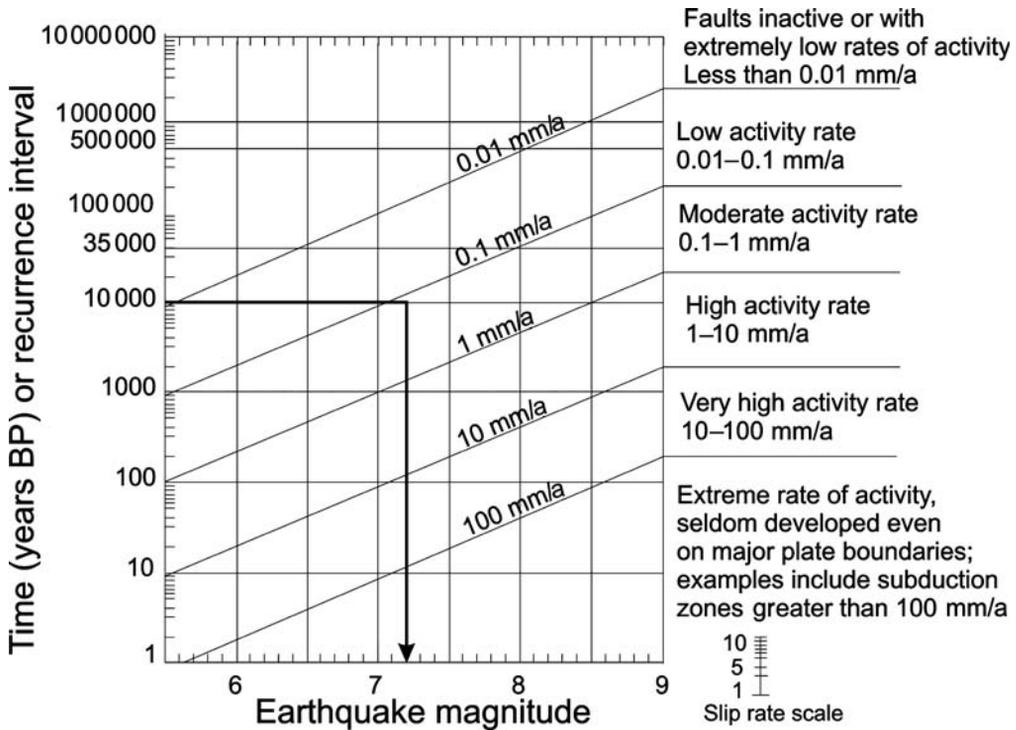
Fig. 14. The relationship between earthquake magnitude and fault offset used to estimate the recurrence time of earthquakes in western North America. After Schwartz & Coppersmith (1984) and Keller & Pinter (1996).
