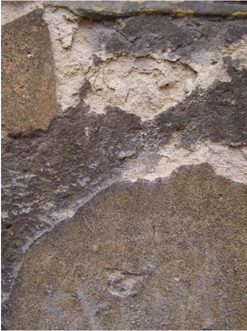
Fig. 7. Multiple gypsum crusts on Jurassic oolitic limestone, Oxford (approximate image width 50 cm).
